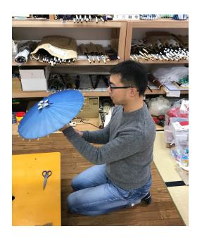
After covering the round tip of the central stick with two pieces of *washi* laying on each other, two thin cords for fixation and one thick cord for decoration are tightly fastened.
