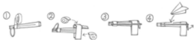
1. Tape two chopsticks, 1cm from the upper part, together with plastic tape and put a rubber band between the chopsticks.
