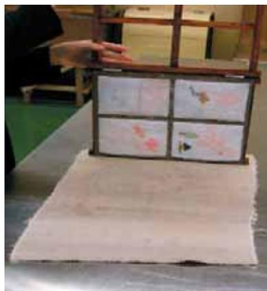
*tap the mold so the dried pulp falls out onto a mat*
