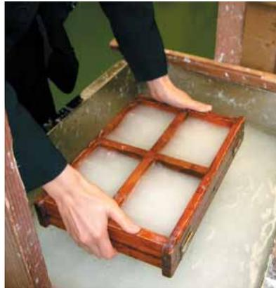
*lifting the mold out of the vat*
